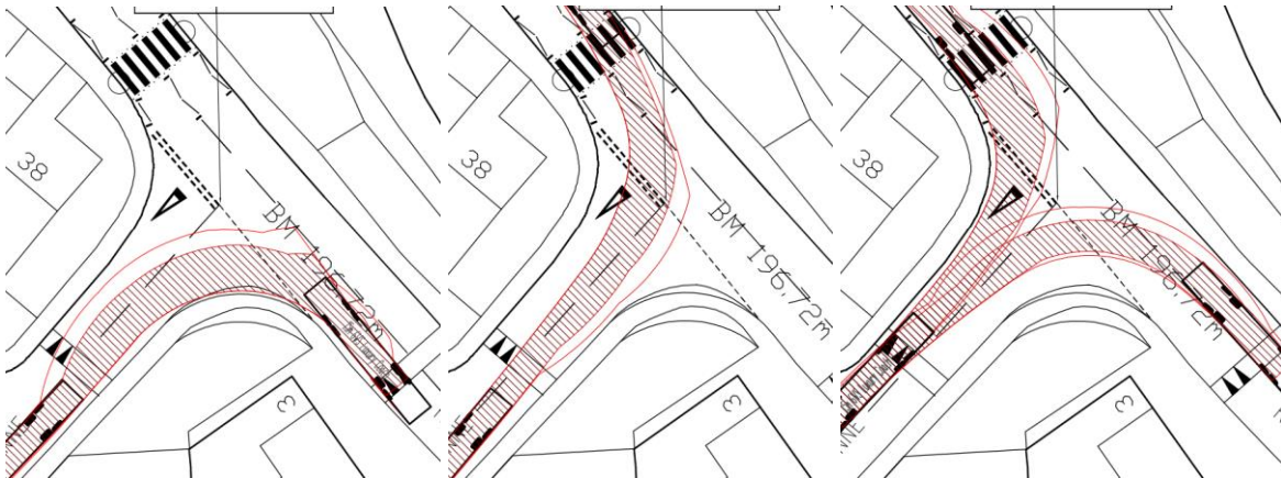
Figure 7 – Swept Path 15m Coach at Proposed 3 Arm Priority Junction
