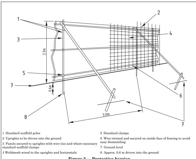
Figure 2 — Protective barrier
