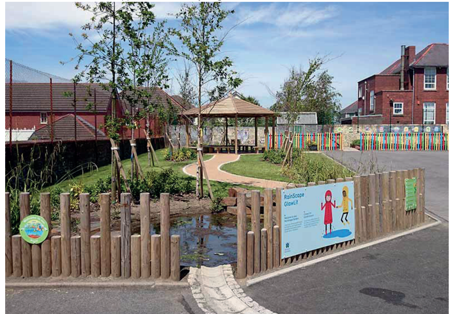
Example - Small pond with overflow via rill to the swale in a primary school
