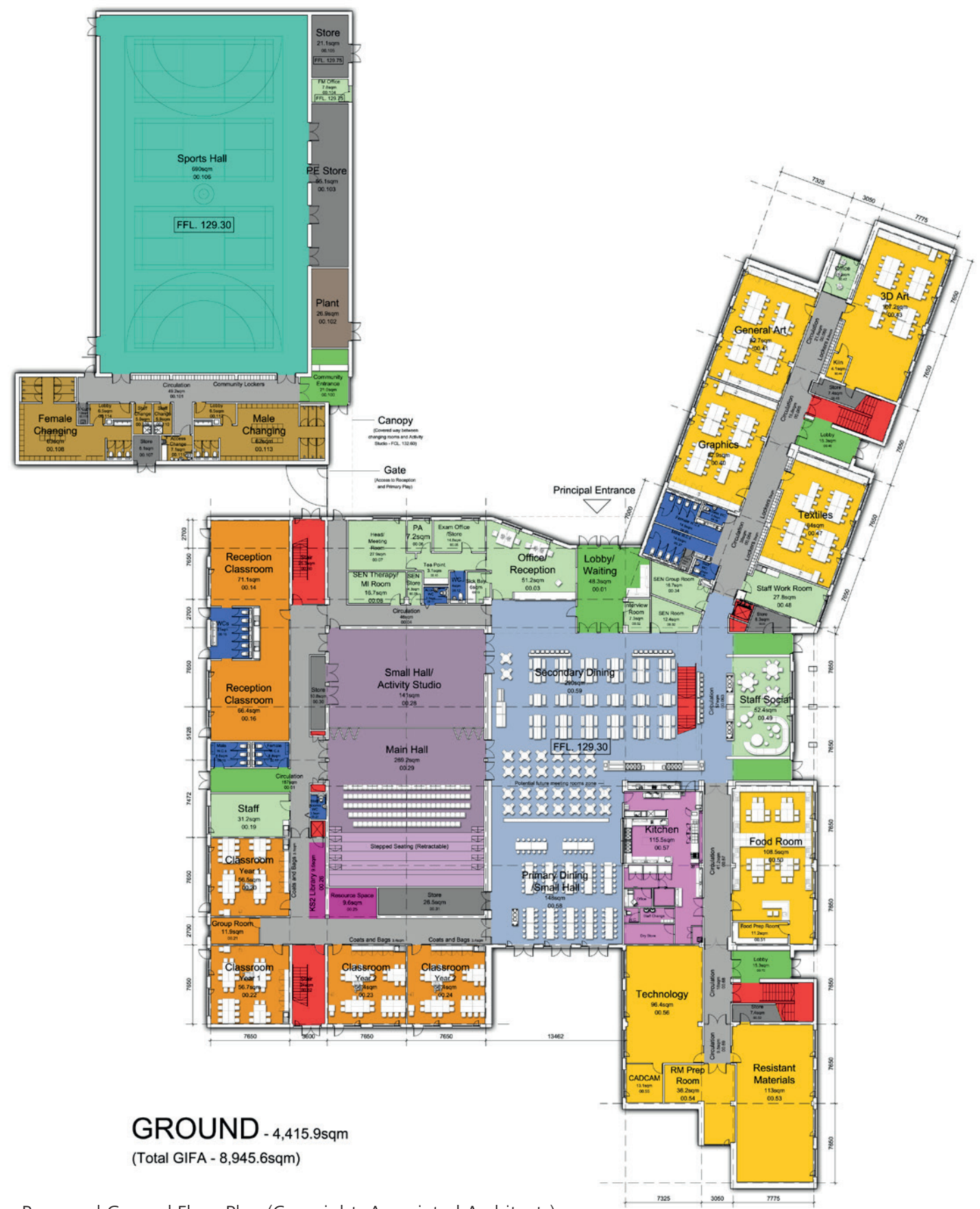
Proposed Ground Floor Plan (Copyright: Associated Architects)
